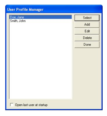
Use the "Select" button to switch to the user highlighted the list. Click "Add" to create a new user. The "Edit" button opens the <u>User Profile</u> for the highlighted user. The "Delete" button permanently removes a user and their measurements.
