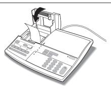
Press the FEED , and cut off the excessive paper.
